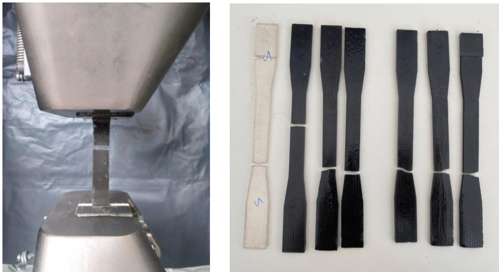
Figure 4.3: Tensile strength testing of the polyester composites with the fracture regions
