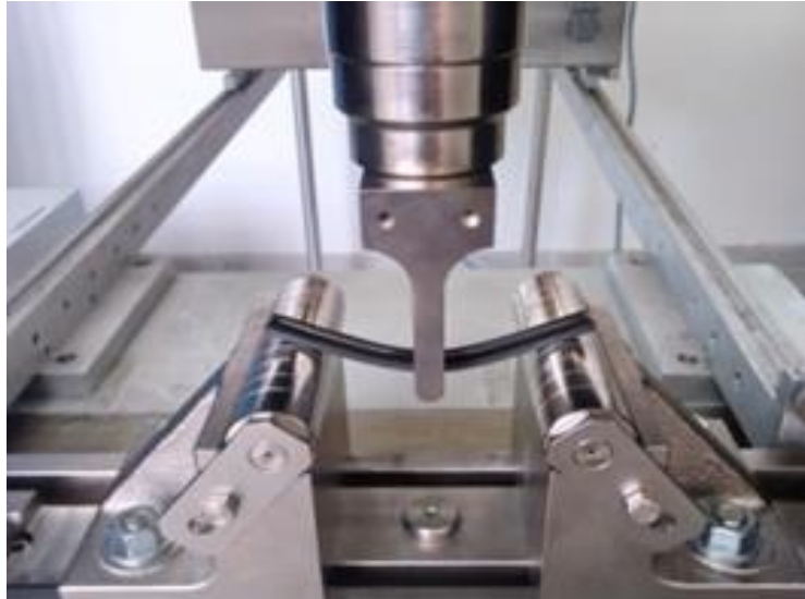
Figure 4.6: The universal three point bending testing machine
