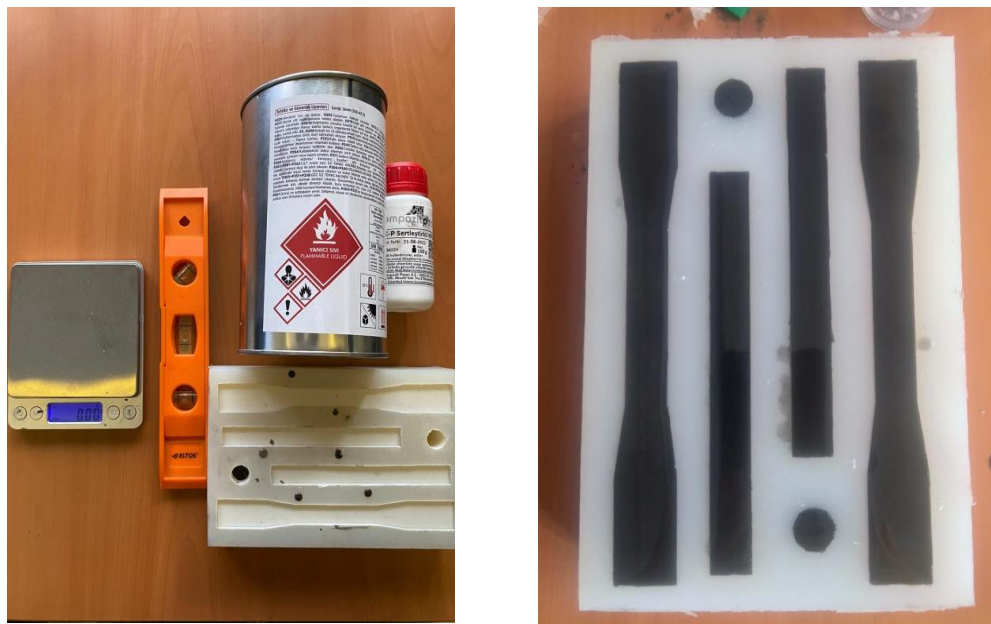
Figure 4.2: Synthesizing the Ti64 powder reinforced polyester composites
