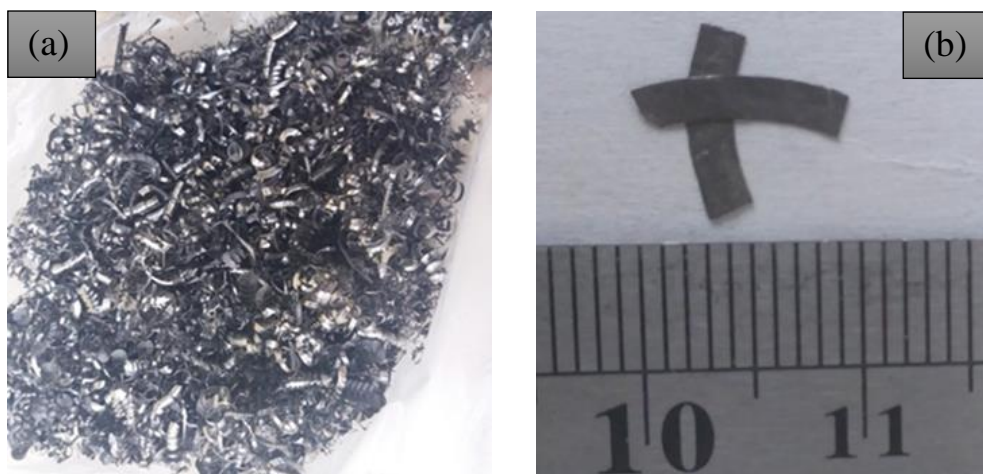
Figure 2.1: Type of machining Ti64 scrap generated (a) as-received chip, (b) pre-milled chip
