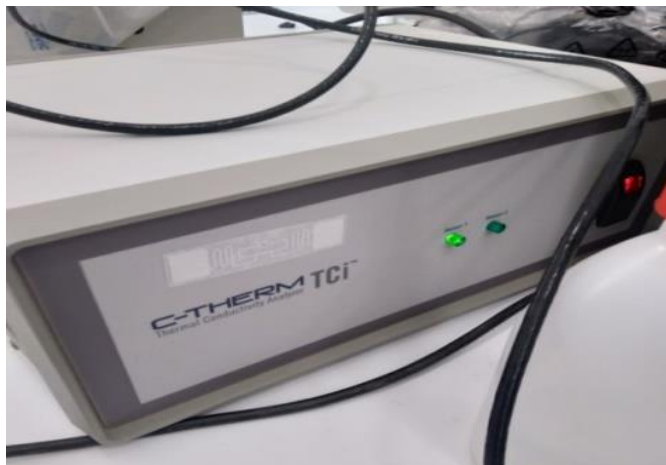
Figure 3.5: C-Therm TCI test machine according to ASTM D 5470
